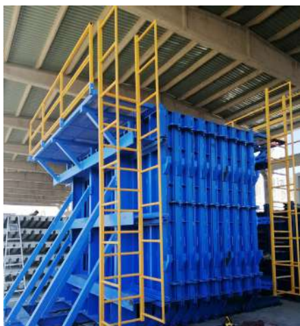
Dohuk / IRAK Moule mural vertical (8 batteries)
